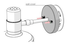
Turn the nut on the side of the knuckle joint to adjust the angle of the shade up or down as desired.
